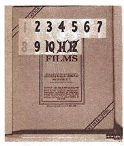
Right: Materials for contact printing guide. Complete setup is shown at right, bottom. Lines are drawn at equal distances on baseboard. Printing frame on the block is placed nearer to or further from lamp according to negative density. Time stays constant.—R. J. Marran.
