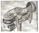
An ingenious new attachment has been developed for 14" drill presses that provides a wide range of speeds for both high and slow speed models. The attachment consists of a heavy casting which mounts in the drill press column together with a cone pulley and two belts. Belt slack is taken up by turning the casting so proper tension is always assured. A range of 12 speeds is available through various combinations. various combinations.
