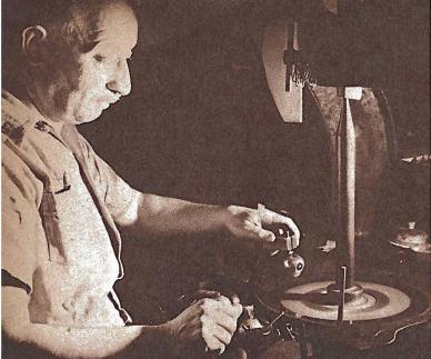
Left: Set in the "dop," a cut diamond is placed on the polishing wheel, which is treated with diamond dust and oil.
