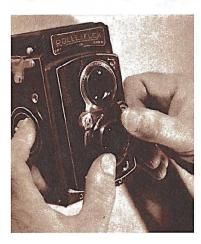
Above: Cellophane held taut in front of the camera lens serves as a fifter. The material must be held flat to avoid lens flate and distortion. Place a equare of, cellophane over the lens then, press over it a ring of brass tubing which normally fits lens mount loosely.—Kenneth Murray.
