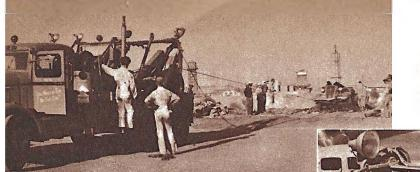
Left: The A-1 Auto Works does a long distance towing job, pulling a large truck out of a deep excavation. The tow truck has two anchors which brace it for jobs such as this one. Below: A closeup of the powerful winches wound with towing cable, on the back of the super tow truck.
