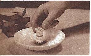
Scaking the heads of a bundle of safety matches in water. Resulting paste is used to prepare other matches.
