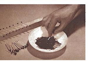
Coating the ends of safety matches with the igniting material so they can be lighted twice.
