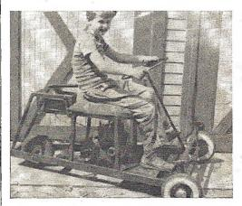
This is a 25-mile-an-hour "put-put" built by Jack Elston, 14 years old, of 2515 Buchanan Street NE., Minneapolis, Minn. "I got interested looking at the midget autos in MI," Jack writes, "so I built my own. All the parts are home made except for wheels, motor, pulleys and belts. It is powered with a 34 h.p. lawn mower motor. A friend of mine is shown on the put-put in this picture." Jack's whizzer looks very workmanlike, and wins him a \$3 Workbench check.
