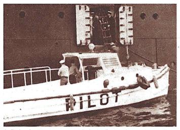
A pilot launch, manned by apprentices, ferries the pilot from the pilot boat which lies at anchor in Ambrose Channel to the incoming liner. Here a pilot enters a side hatch.
